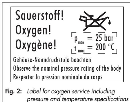
**Fig. 2:** Label for oxygen service including pressure and temperature specifications
