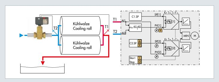
flow rates provided. The task was to develop a compact control unit with a sufficient level of control accuracy to fulfil two assignments: control the cooling water's differential temperature upstream and downstream of the rolls to between 2 and 4 Kelvin and control the cooling water's return flow temperature to a maximum value. Such a solution was not available on the market off the rack. Consequently,
