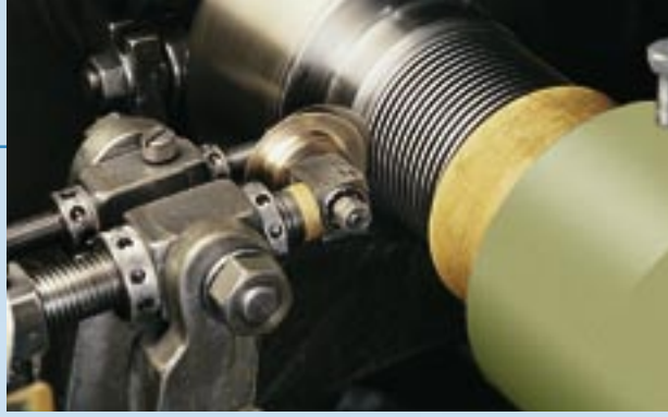
SAMSON manufactures its own standard bellows from stainless metal sheets on self-developed machines.
