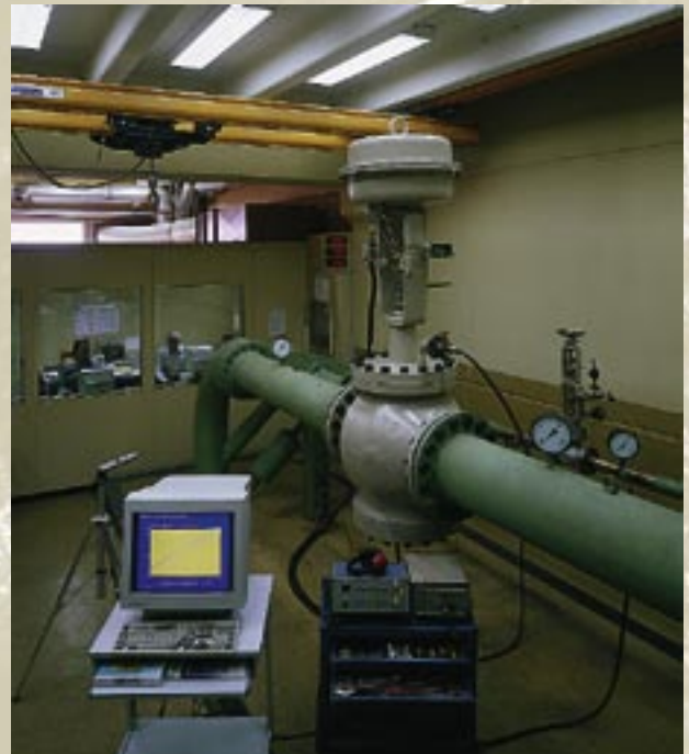
Automated measurements of valve-specific parameters can be performed across the entire travel range.
