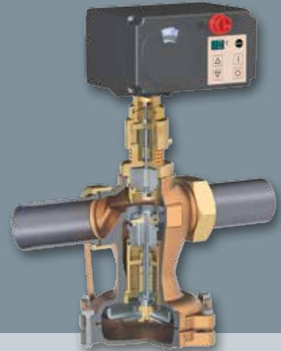
The principle of operation employed by self-operated regulators is both simple and effective. They do not need any additional energy supply as they draw the required actuating force from the process medium they control. The pressure to be controlled is routed onto an actuator diaphragm through a control line. In pressure-balanced regulators, only the force of the set point spring opposes the actuating force. Any change to this balance
