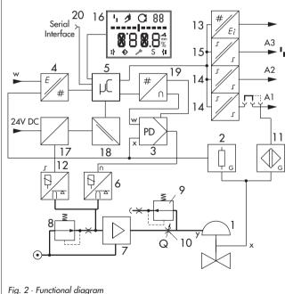
Control valve 2 Travel sensor PD controller
