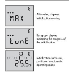
After a successful initialization, the positioner runs in control operation indicated by the C control symbol.
