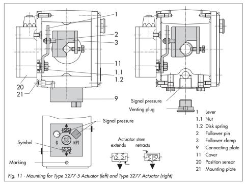
Place the lever (1) in mid-position and hold it in place. Screw on the nut (1.1).
