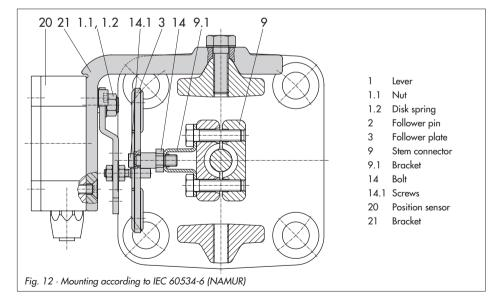
For other actuator sizes or travels, select the lever and pin position from the travel table on page 13. Lever **L** and **XL** are included in the mounting kit.
