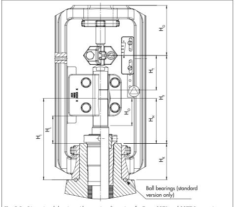
Fig. 5-5: Dimensional drawing with mounting dimensions for Types 3271 and 3277 Pneumatic Actuators
