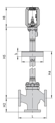
Type 3246 as three-way valve  $\cdot$  NPS  $\frac{1}{2}$  to 6 (DN 15 to 150), Class 150 and 300 (PN 16 and 40)
