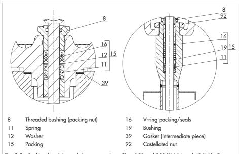
Fig. 9-3: Packing for globe and three-way valves, Class 150 and 300/PN 16 and 40 (left) · For globe valve, Class 600 and 900/PN 100 and 160 (right)
