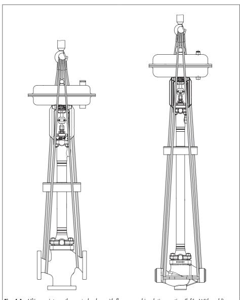
Fig. 4-1: Lifting points on the control valve: with flanges and insulating section (left) · With welding ends and insulating section (right)
