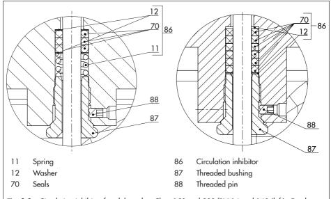
Fig. 9-2: Circulation inhibitor for globe valve, Class 150 and 900/PN 16 and 160 (left) · For threeway valve, Class 150 and 300/PN 16 and 140 (right)
