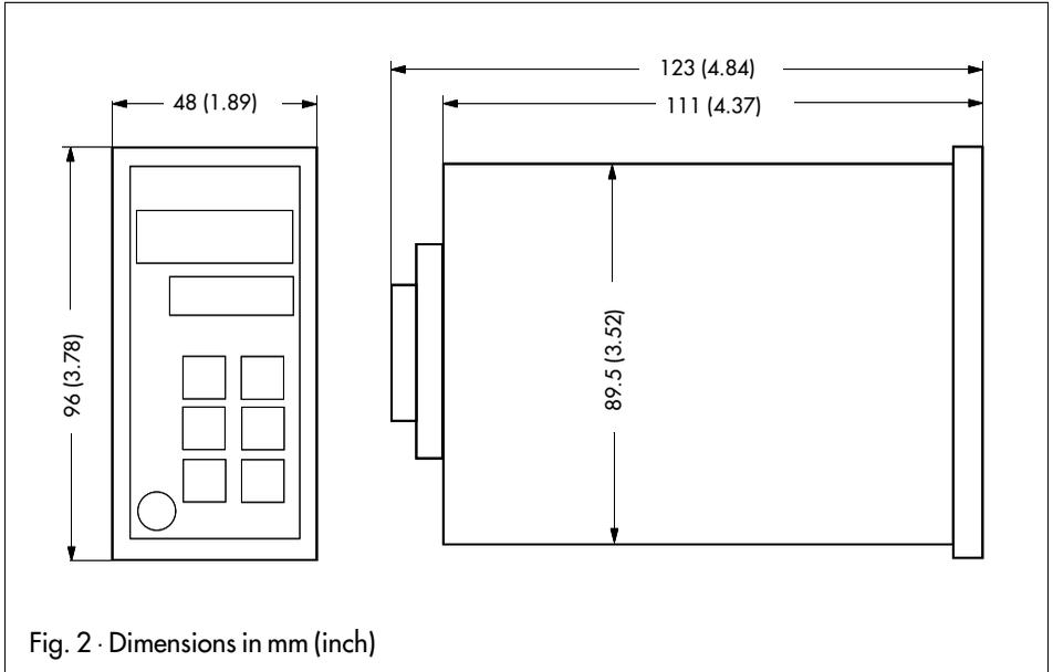
Fig. 2 · Dimensions in mm (inch)
