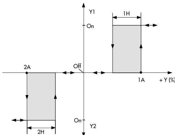
Fig. 11 · Switching 2\*on-off output with **Y1 = 7** and **Y2 = 6**
