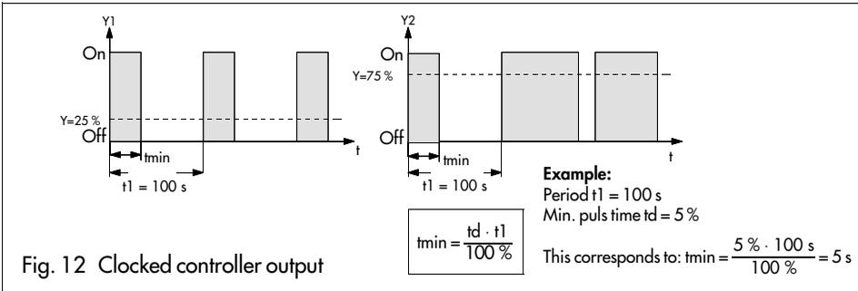
Fig. 12 Clocked controller output
