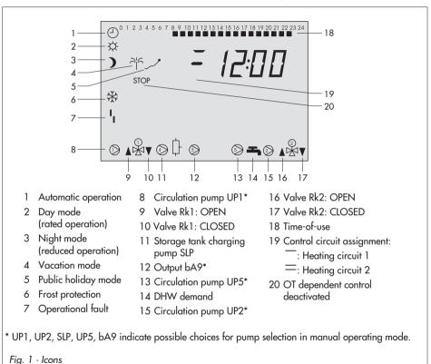
The controller status can be displayed in operating level (-> section 1.4).
