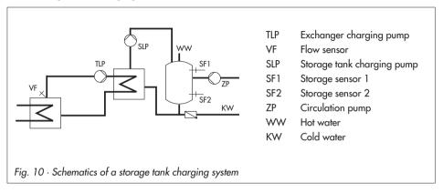
The controller begins charging the storage tank when the water temperature measured at sensor SF1 falls below the DHW temperature set point by 0.1 °C. If the flow temperature in the system exceeds the required charging temperature, the controller tries to reduce the flow temperature in the heating circuit for up to 3 minutes before the exchanger charging pump is activated together with the storage tank charging pump.
