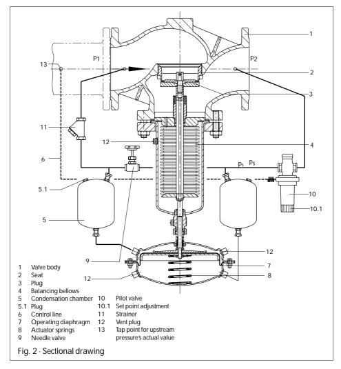
the actuator spring force has more effect. The valve plug also moves in the closing direction until the set point is reached.
