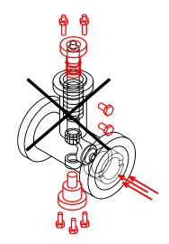
The lateral screw is not a port sniffer. It serves as a blow out for the shaft and therefore must not be removed during the operation in the pipeline or in the system.
